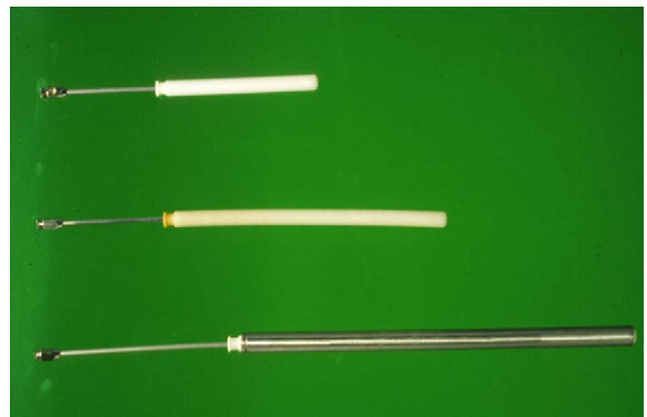
Fig. 2. The transcervical stainless steel catheter (Lima A/S, Sandnes, Norway) comes in three sizes: large (bottom, with a stainless steel guiding tube), medium (middle), and small (top) with plastic guiding tubes. Catheter dimensions: large, medium, and small dogs: length: 46, 31 and 21 cm; diameter of main part of catheter: 3, 3, and 2.8 mm; length of smaller neck 4.5, 4.3, and 2.4 cm; neck diameter: 1.2, 1.2, and 1.0 mm; and ball tip diameter: 1.8, 1.8, and 1.3 mm. The length of the guiding tubes are 31, 22, and 12.5 cm, respectively, and the external diameter is 9 mm.
